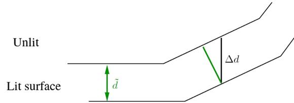
Figure 14: Adjusting the depth offset: as the depth of the lit layer  $\tilde{d}$  should be measured perpendicularly to the surface, and not along the viewing direction,  $\tilde{d}$  should be scaled accordingly to get the proper offset  $\Delta d$ .
