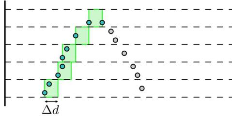
Figure 15: Shadow map generation: using the depth peeling approach, all points within the green boxes of width  $\Delta d$  are marked as lit.
