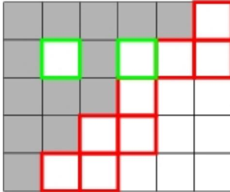
Figure 2: Closeup view of the rendered surface’s border. Pixels that have been filled in the first pass (point rendering) are shown in grey, background pixels in white. All background pixels close to a filled pixel are framed. Green frames indicate holes in the surface rendering and the respective pixels have to be filled. Red frames indicate pixels that are beyond the silhouette of the object and must not be filled.
