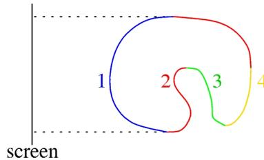
Figure 8: 2D illustration of depth peeling: visible layers of geometry are extracted from front to back. First layer is shown in blue, second in red, third in green, and fourth in yellow.
