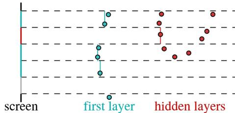
Figure 9: When projecting first layer (blue) in point cloud representation to the screen, the layer exhibits holes such that hidden layers (red) or the background (grey) become visible.
