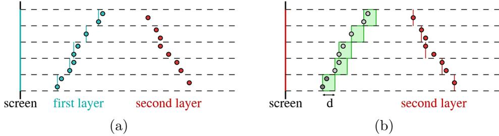
Figure 11: Depth peeling for transparent rendering: (a) first rendering pass records closest points and their depths; b) second rendering pass again records the closest points and their depths, but ignores points less than  $\tilde{d}$  away from the reference depths obtained in the preceding run.
