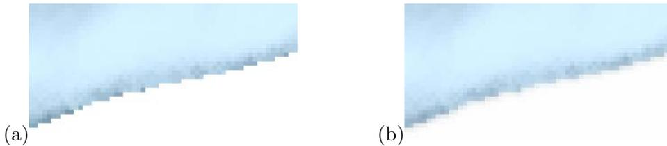
Figure 7: (a) Close-up view on skeleton hand data set exhibits aliasing artifacts along the silhouette of the object. (b) Anti-aliasing by blending with high-pass-filtered depth buffer texture.
