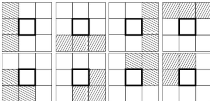
Figure 3: Filters with size  $3 \times 3$  for detecting whether a background pixel is beyond the projected silhouette of the object. If one of the eight masks matches the neighborhood of a background fragment, it is not filled. White cells indicate background pixels, dark cells may be background or non-background pixels.
