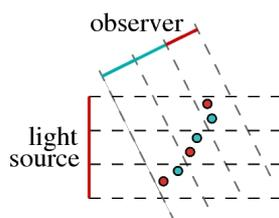
Figure 13: Inconsistent shadow map in case of high point density: marking only the closest points to the light source as lit, leaves unlit points on the same surface part. The unlit points become visible when positions of observer and light source do not coincide.
