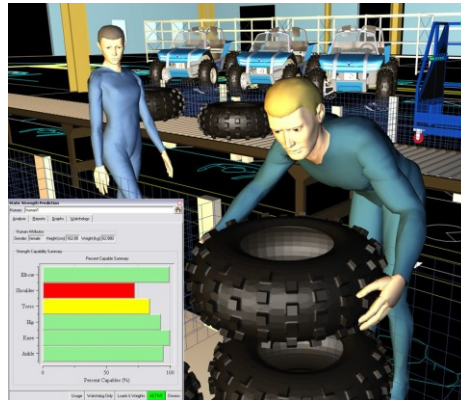
Fig. 2. Ergonomic report of RULA in the DHM "Jack" [12]. The report is displayed in a 3D scene. Here, a static pose of a male worker is considered. The analysis results are color coded for several body parts (e.g., the elbow or the shoulder), as shown in the bottom left corner.
